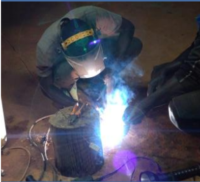
Welding repair strap at local workshop
