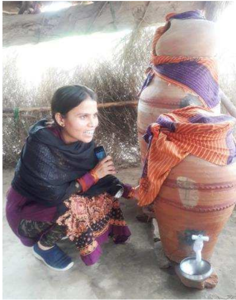
Nadi filter (water fed through upper pot into filter pot then discharges into urn)
